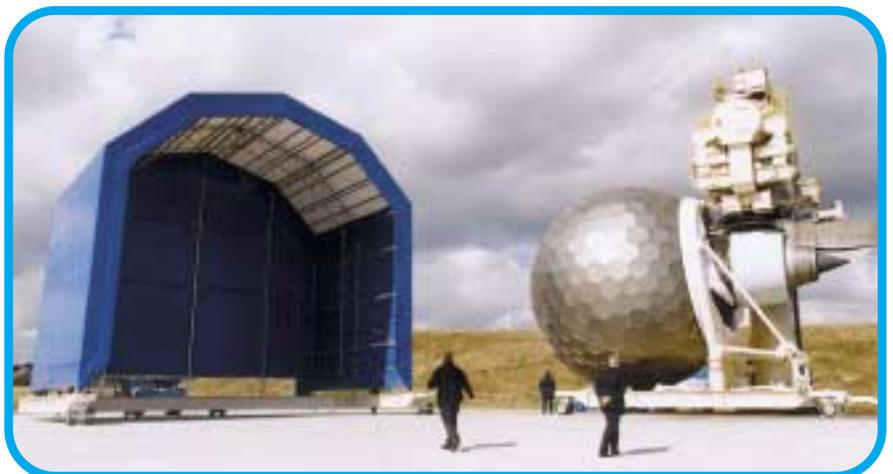
*Trolley allows for the structure to be moved quickly if the weather changes*
