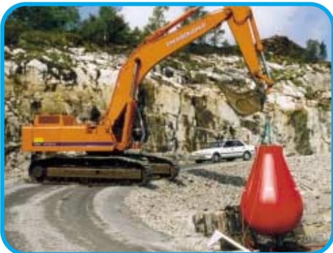
*New 10 ton Aquaweight undergoes testing and passed, proving the strength of Rubb PVC*
